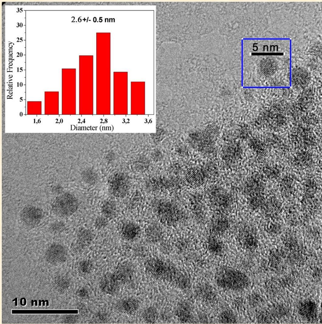
Typical TEM and HRTEM images of the Pd nanoparticles in [Emim][BF<sub>4</sub>] and a size histogram of the Pd-NPs.
