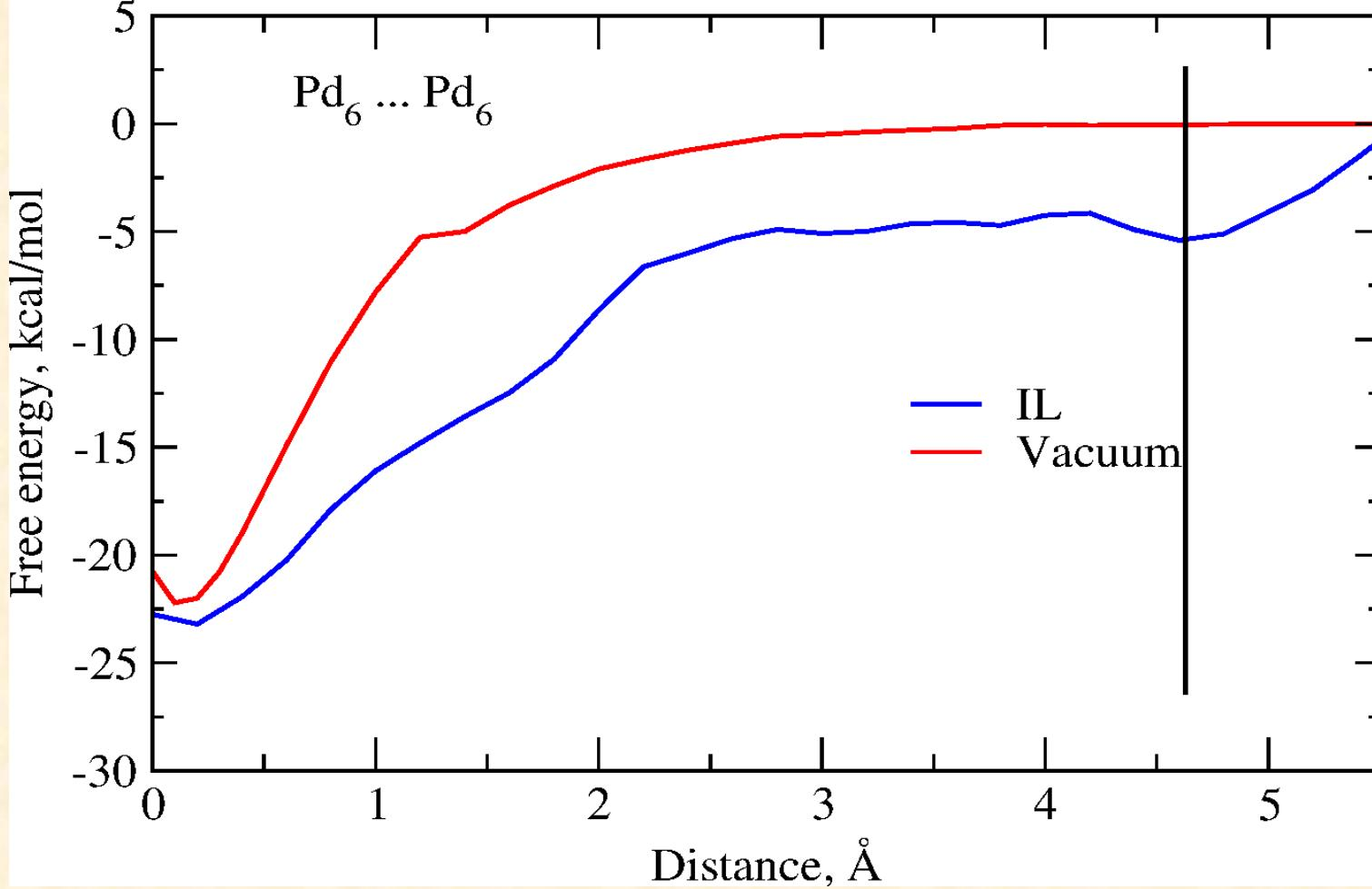
Potential of mean force to displace two Pd<sub>6</sub> clusters in vacuum and in the ionic liquid. Distances are given relative to the minimum energy interaction distance
