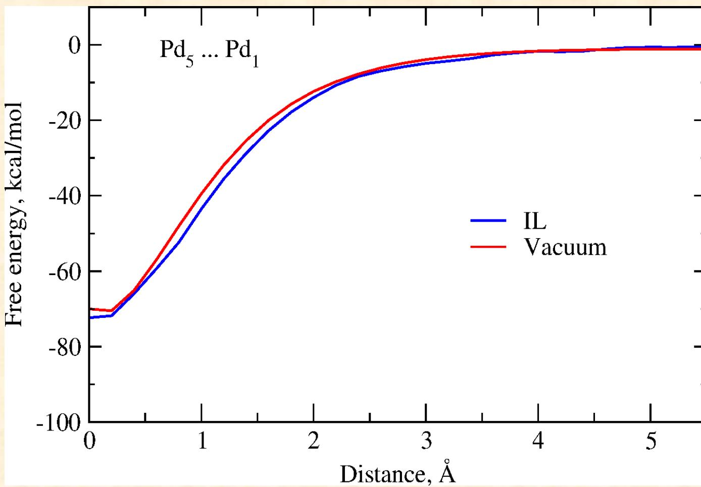
Potential of mean force to displace a palladium atom from the Pd<sub>6</sub> cluster in vacuum and the ionic liquid. Distances are given relative to the minimum energy interaction distance
